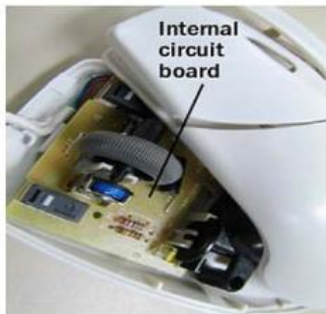
Figure 4. Typical internal circuit board of a mouse
